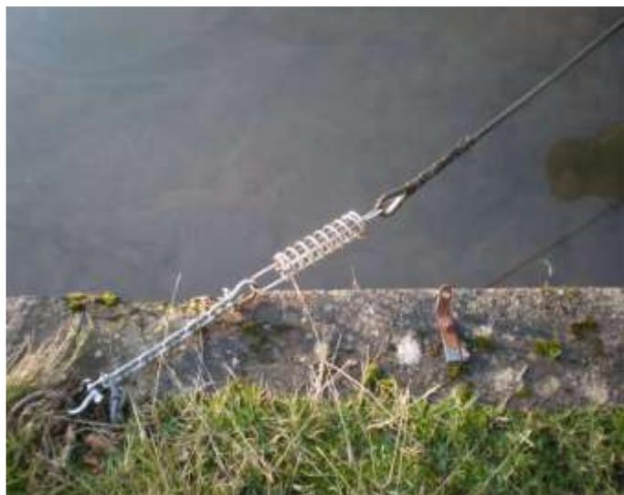
extensions (right) on my lines which with good fenders allows the boat to move within limits. It
