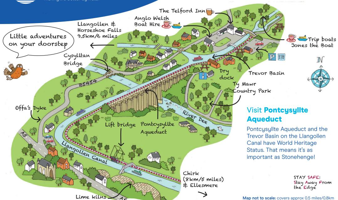
Thomas Telford and William Jessop designed Pontcysyllte Aqueduct to carry the Llangollen Canal across the Dee Valley. Completed in 1805, it's a cast iron trough supported on giant stone pillars 39 metres (127 feet) above the river. It's one of the most awesome engineering feats on the canal network.
