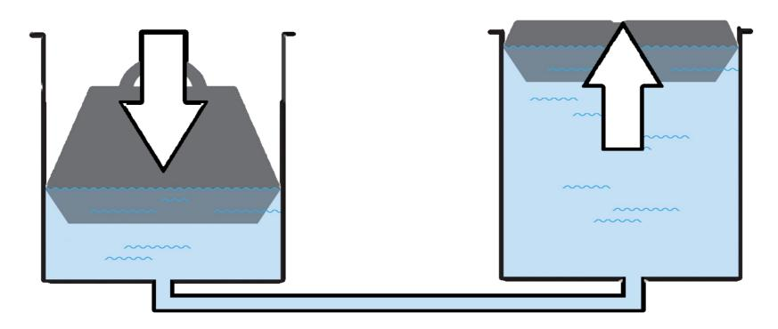
Connecting syringes together you can transfer force from one syringe to the other.
