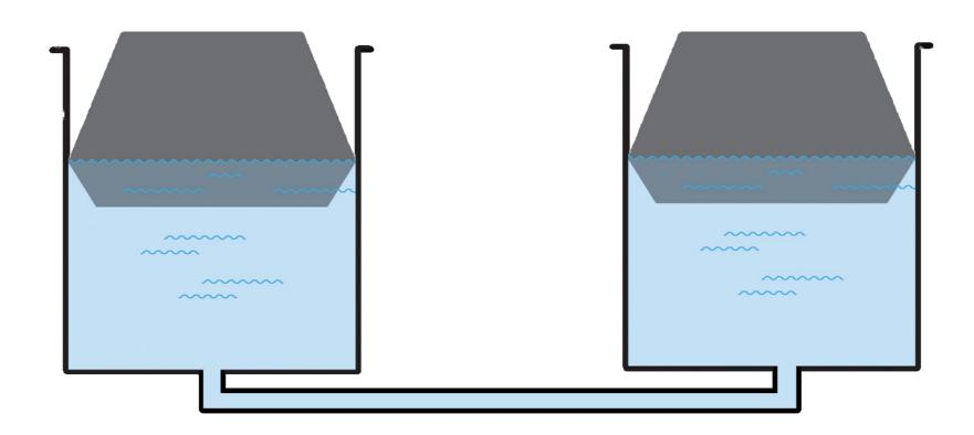
Using a fixed volume of water we can transfer forces from one place to another.
