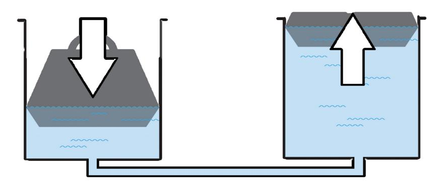
If we push down on one side the liquid flows through the pipe and pushes up on the other side Remember water always takes up the same amount of space
