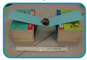
Place the small weights onto the strip of card until your card falls into the gap. How much weight did it hold?
