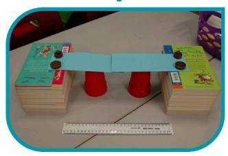
Lay a strip of card or ruler on each pile of books, with 5cms of card resting on the pile, and the rest of the card laying over the plastic cup.
