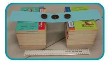
Place the small weights onto the strip of card until your card falls into the gap. How much weight did it hold? Test your bridge by changing the amount of card used and the width of the gap, using the chart on the next page.
