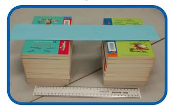
Place the books in two piles of equal height and ensure that there is a gap of 10cms between the two piles.
