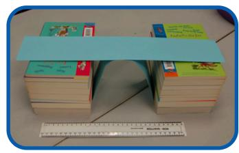
Place the books in two piles of equal height and ensure that there is a gap of 15cms between the two piles. Cover the gap between the two piles of books with one strip of card. Place another strip in an arch shape between the two piles of books. Make sure the top of the arch meets the underside of the cover.
