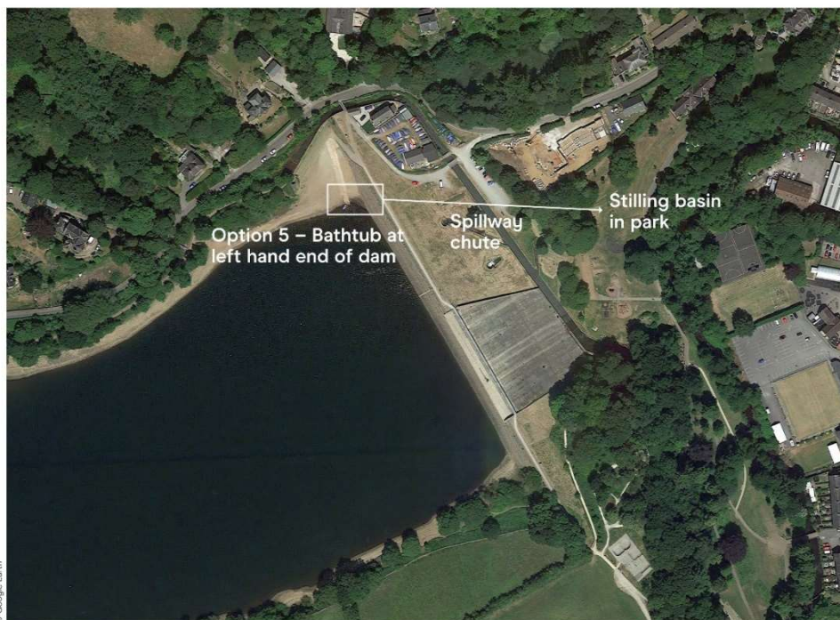
Figure 11: Example of bathtub spillway within reservoir
