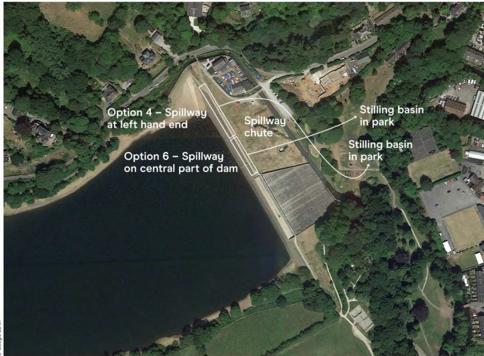
Figure 9: Diagram to indicate locations of spillway options on the dam
