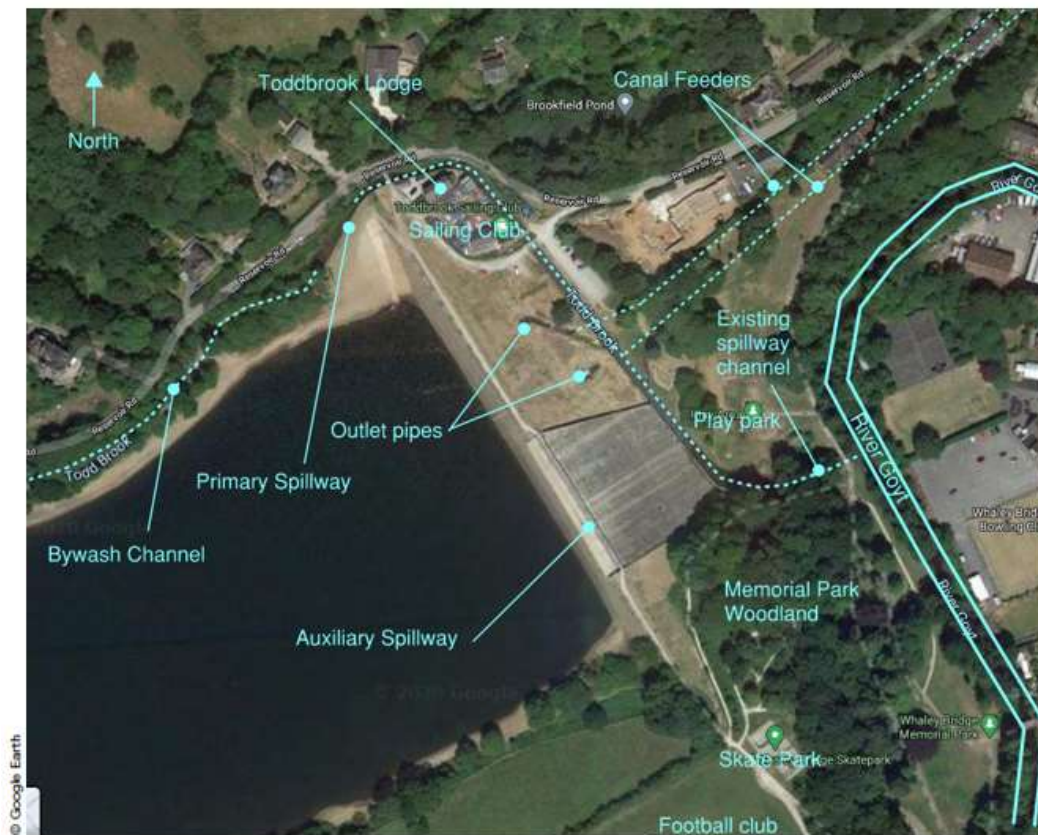
Figure 2. Toddbrook Dam key features
