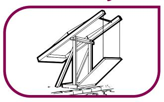
Manual lift bridges have a chain which hangs from the 'balance arm'. When the bridge is open care needs to be taken to ensure the bridge doesn't fall back down again. Sometimes there is a special mechanism and sometimes a person needs to sit on the balance arm until the boat is clear.
