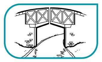
Split bridges are a type of cantilever bridge and were often built next to locks so that the boater could get from one side of the lock to the other. As the horse pulled the boat out of the lock the towrope could pass through the gap in the middle of the bridge.
