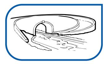
This is a special type of arched bridge, specially made for canal boats being towed by horses.
