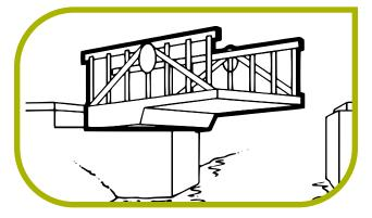
Swing bridges need to open to let boats through. They swing on a pivot until they are parallel with the bank. Manual swing bridges can usually be moved with a good push after unhooking a retaining chain – they are likely to be used for pedestrians only.
