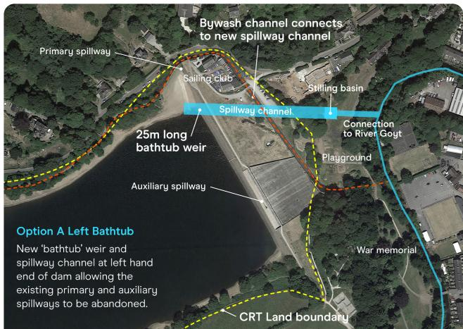
"Under either option, the existing auxiliary spillway (damaged last summer) becomes redundant and replaced with a grassy slope. The smaller original primary spillway near the Sailing Club will also be de-commissioned.
