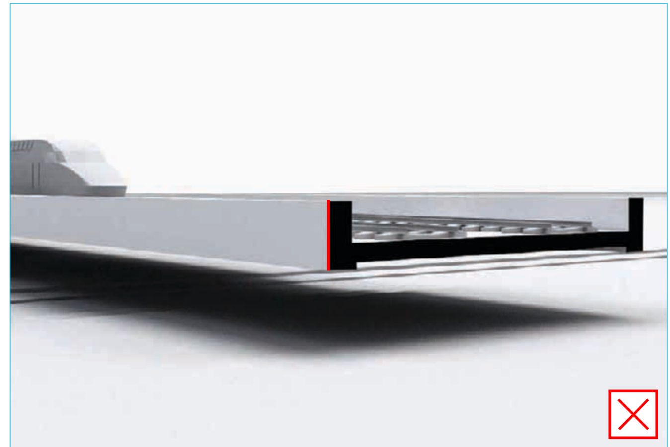
Fig.B11.1 - Rectilinear edge condition creates heavy appearance
