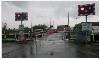
Sandfield Bridge showing poor sight of oncoming vehicles over the bridge, no hatching and adjoining track junction on left
