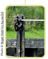
A **gear mechanism** is used to open and close the paddles.
