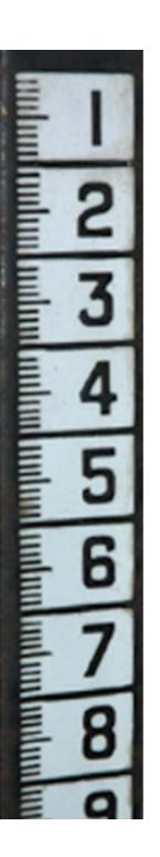
A gauging rod was a stick with measurements marked on it, used to measure the freeboard – space between the water level and the gunwale of the boat.
