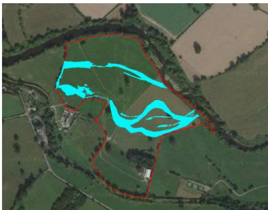
Figure 3.12. Backwater feature inundation from ditch blocking via chute activation, estimated flow in ditches.
