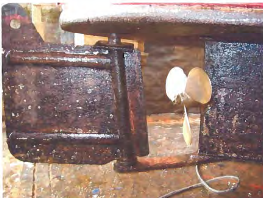
Figure 4.3 Narrow boat with propeller and rudder configuration
