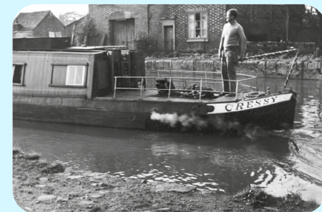
A wooden horse-drawn narrow boat Cressy converted into a houseboat by Rolt
