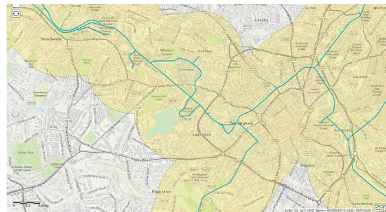
Illustration of the buffer of one kilometre either side of the centreline of the waterway network owned and / or managed by the Trust created using GIS software
