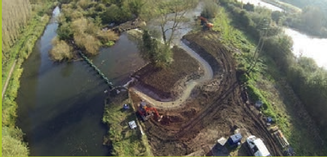
Fish bypass around Dog Head Stakes weir
