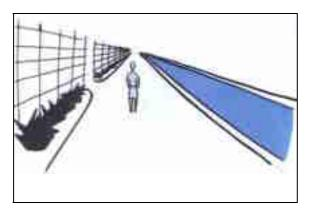
**Figure 6.9**: An example of the fencing or railings combined with dense planting allowing glimpses through but make it difficult to climb.
