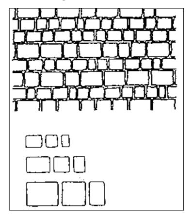
**Figure 9.5**: Sketch showing different sized concrete brick paving blocks that can be used together to give a coursed random appearance.
