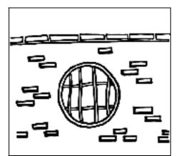
**Figure 6.10**: An example of walling with "feature" railing panels allow limited views through.
