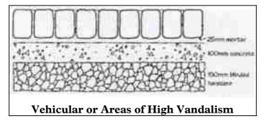
**Figure 9.3**: Sketch cross sections illustrating different laying and jointing methods for stone setts.
