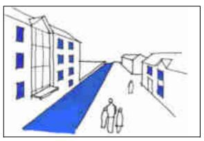
**Figure 7.3**: Sketch examples of towing path environments where the towing path width and the scale of built development maintains the traditional waterside enclosure without being oppressive and provides the towing path user with good visual appreciation of their surroundings.
